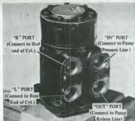
Fig. 6—View of steering control valve identifying inlet and outlet ports with locations and functions.
