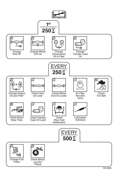
Note: Engine oil and filter service interval can be extended. See Engine Manual for details.
