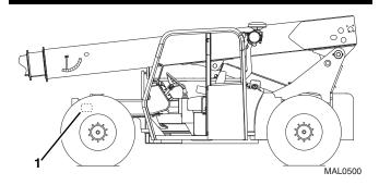
Before ordering parts or initiating service inquiries, make note of the machine serial number. The machine serial number plate (1) is located as indicated in the figure.
