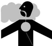
Generator exhaust contains poisonous CO (carbon monoxide) that can cause serious injury or death.
