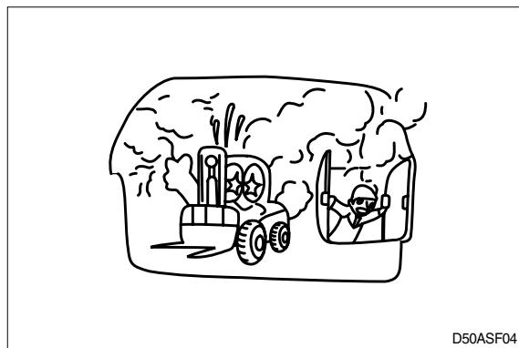
**⚠** Be particularly careful when removing the radiator cap and the hydraulic oil tank filler cap, if this is done immediately after using the machine, there is a danger that boiled oil may spurt out.
