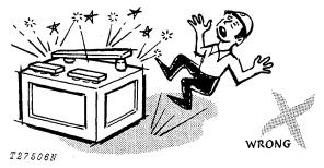
Don't check battery charge by placing metal objects across the posts.
