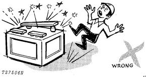
Do not check the battery charge by putting metal objects across the posts.
