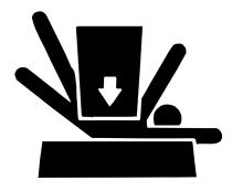
If you must work on a lifted machine or attachment, securely support the machine or attachment.
