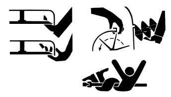
Keep hands and feet away while machine is running. Shut off power to service, lubricate or remove mower blades, augers or PTO shafts.
