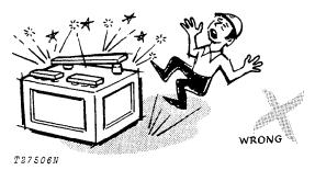
Do not check the battery charge by putting metal objects across the posts.
