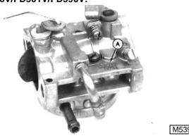
The carburetor serial number (A) is located on the top of carburetor.
