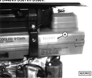
The engine serial number (A) is located on the side of the cooling air duct.
