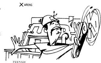
If you must work on the machine with the engine running, ALWAYS USE TWO service technicians. One must be at the controls. The other must be within sight of the operator.
