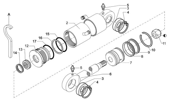
(one cylinder side with end stroke dampening)
