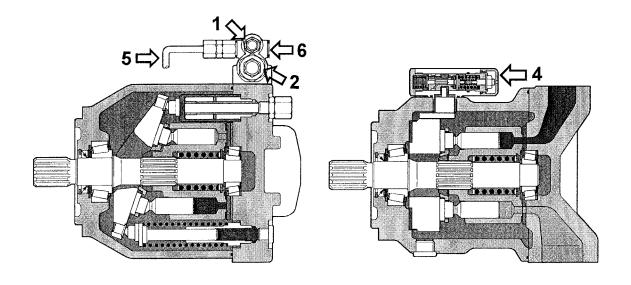
The PLS valve compensates pressure peaks, which can create a short change of the pressure difference, provided that the  $\Delta p$  of the pump regulator is set by 5 to 8 bar lower than the  $\Delta p$  of the PLS valve.
