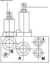
setscrew pressure reducing valve pilot pressure: 32 bar
