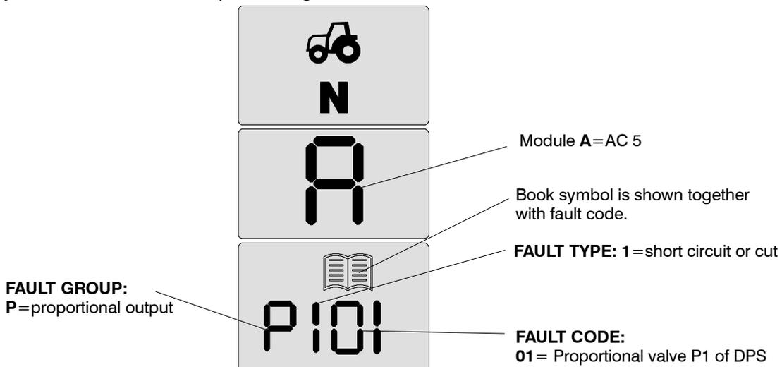
**IMPORTANT!** Escaping from the fault code mode is done by switching off current with the starter switch, when the fault codes exit from the display block.
