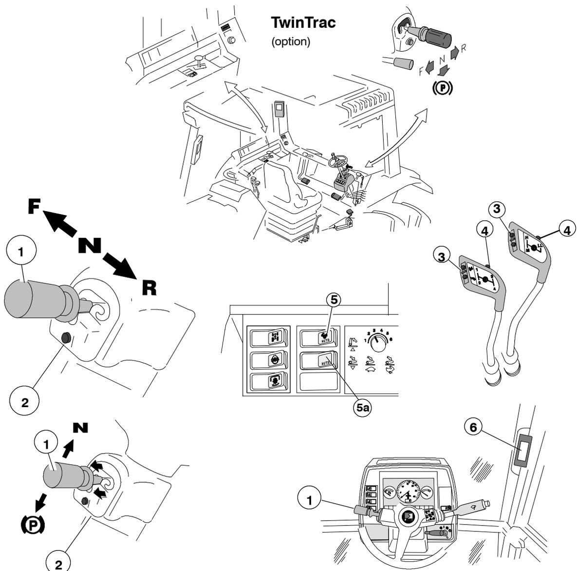
1. Reverse shuttle lever/hand brake lever on the LH side of the steering wheel (or alternatively on the RH side). The parking brake must always be engaged, when the tractor is parked.
