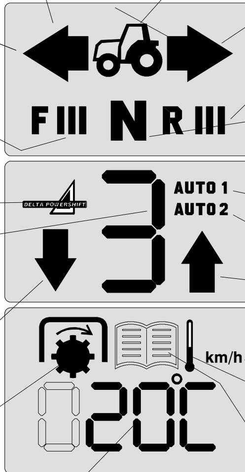
Outdoor temperature when the tractor is stationary. Driving speed when the tractor is in motion (accuracy one decimal □ 15 km/h. No decimal at greater speeds). Numbers show also fault codes. In the test mode is shown a point, which is tested or reset.
