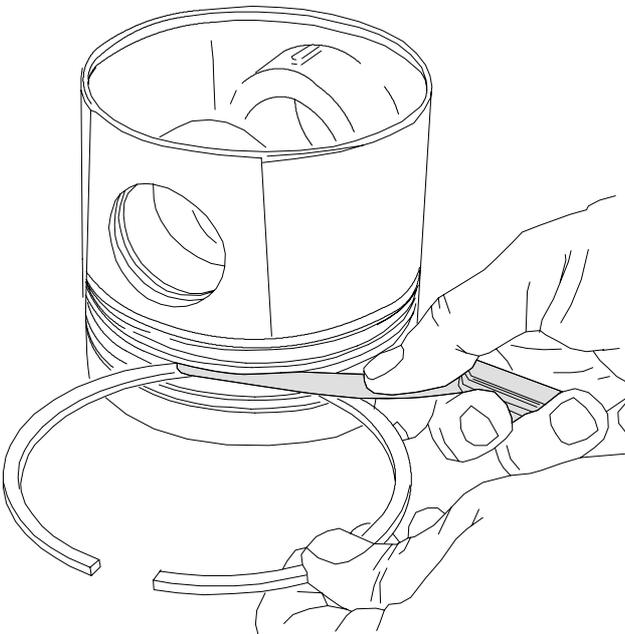
2. Clean the piston ring groove and measure the piston ring clearance, which must not exceed **0,15 mm**. Determine whether too large a clearance is due to worn rings or a worn groove. Change worn parts.
